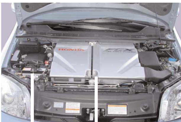
12V Battery Power Control Unit
