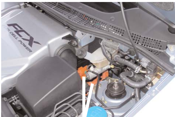
High-Voltage Cables (driver's-side under-hood view)
