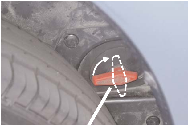
Manual Hydrogen Shut-Off Valve (Turn 1/4 turn clockwise to stop the flow of hydrogen.)
